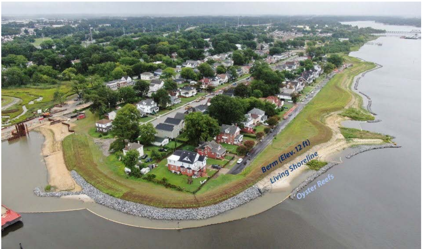
Adaptation tools are often most effective when used together. This Norfolk neighborhood employs a number of flood mitigation techniques, including an elevated berm and living shoreline.
